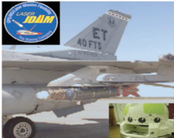
Laser-guided MK-82 scores direct hit against a moving target during tests at Eglin AFB.
