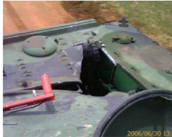
Affordable hit-to-kill accuracy minimizes collateral damage; the photograph shows the hole made in the target by a (nonexplosive) weapon.
