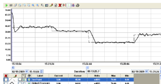
Fig. 15. Experimental result for a PIV of 2 inch diameter located in Florencia (Caquetá, Colombia). We use multiple operation points with S=10 , N_1=1 , N_2=1 , N_3=4 , and C=0.001 . The solid line is A_{PIV} and the dashed is the reference.
